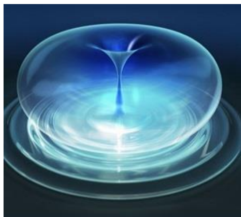
Illustration of an imploding cavity in a liquid under cavitation
